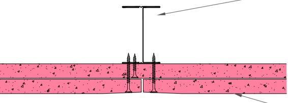
2x15mm Siniat GTEC Fire Board fixed with SPEEDLINE Drywall Screws at 300mm centres (200mm centres at external angles). Ref to table for fixing length.
